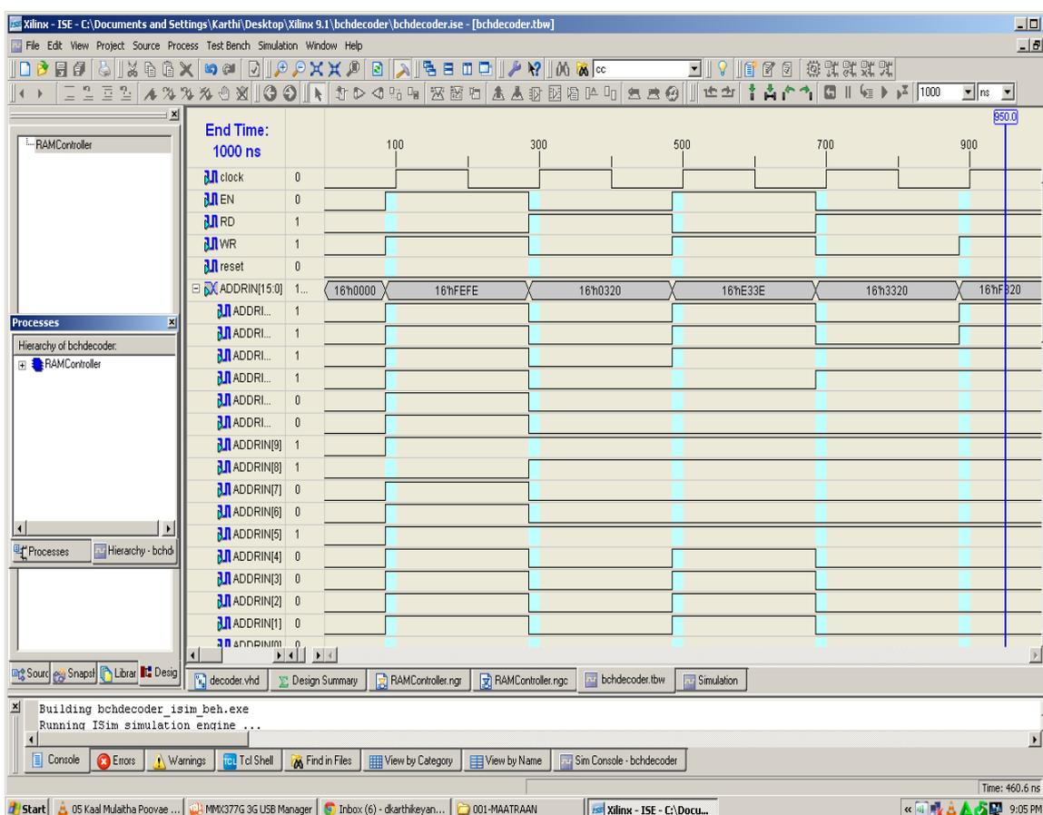
Figure.4 Binary BCH code and test bench wave form
