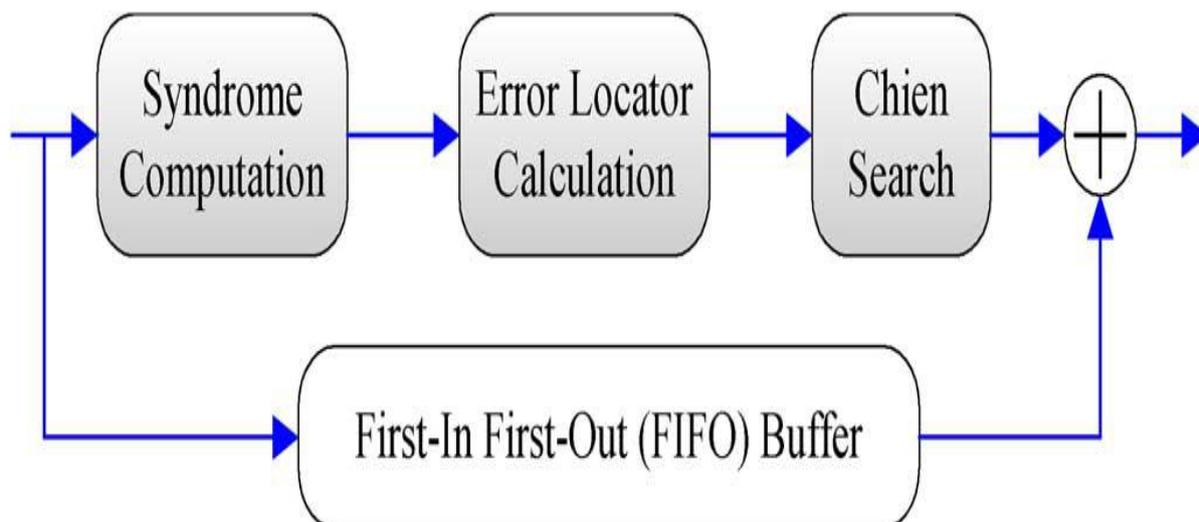
Figure.2 Binary BCH code decoder structure.
