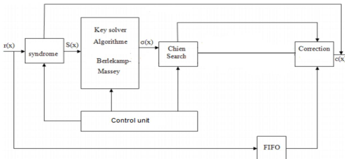
Figure.2 Digital circuit for BCH decoder
